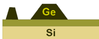
Figure 14. A schematic diagram of the formation of Ge islands on Si(111).
